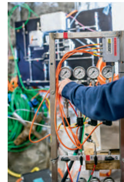
Project manager Florian Amann. One turn is all it takes to adjust the water pressure in a borehole.
